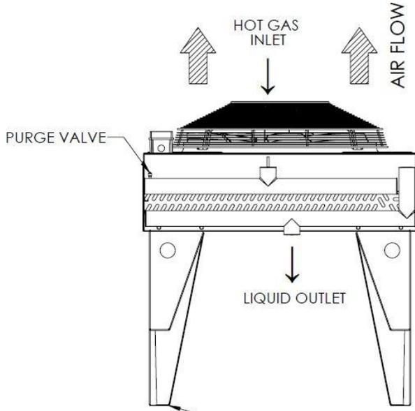
EXTENDED LEGS AVAILABLE AS AN OPTIONAL EXTRA FOR MODULES QAC 3500 THRU 7500 AND MULTIPLE MODULES
