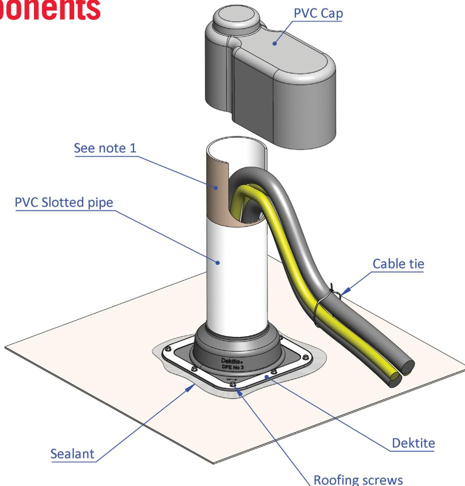
Note 1 : Optimum performance is achieved when PVC solvent adhesive is used on these parts
