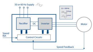
Figure 11: Operation with inverter
