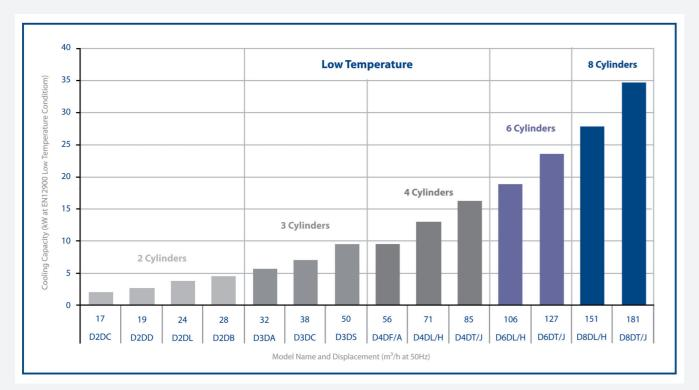
Figure 4: Low temperature coverage from 2 – 35kW cooling capacity
