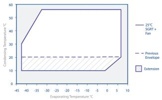
Figure 7: Medium / High temperature R404A envelope for Discus® compressors with large motor
