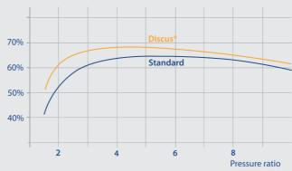
Figure 10: Typical Discus® and standard reed valve compressor isentropic efficiencies at low condensing pressures below 20°C
