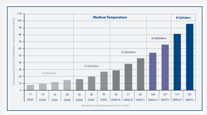
Figure 3: Medium temperature coverage from 7 – 95kW cooling capacity
