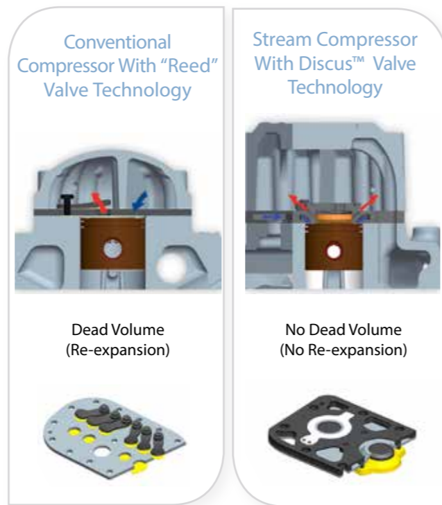
Figure 2: Key difference between conventional reed and Discus valve technology
