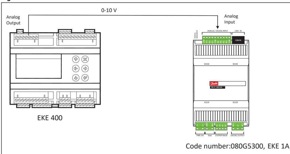
Figure 35: Electrical connection
