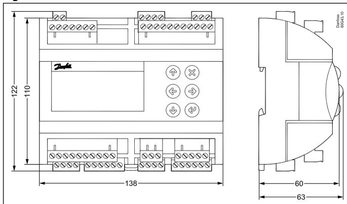
For DIN rail mounting only (IP 20)
