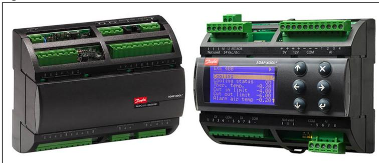
For industrial refrigeration applications the Danfoss EKE 400 can control the operation of the valves and the fans for evaporators to achieve optimal cooling mode and defrost sequence for an efficient, safe and trouble-free operation of the evaporators, complying with IIR<sup>(3)</sup> safety recommendations for hot gas defrost.
