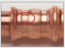
To confirm that the press cycle was completed properly, an RLS witness mark appears within each press band (one on each side of the fitting). If the RLS mark is not visible, the fitting must be re-pressed, or removed and replaced.
