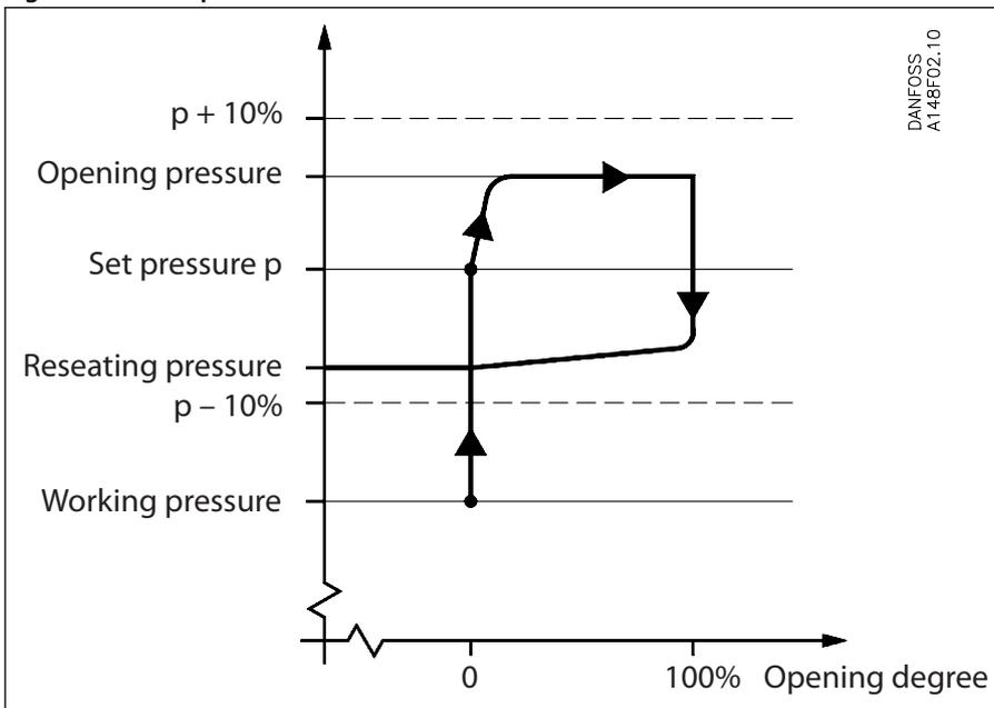
SFV is designed as a standard safety relief valve (DIN 3320), which are recommended for refrigeration plants. On a rise in pressure above the set pressure, the safety relief valve will initially start opening slightly, to minimise the outlet of refrigerant. If the pressure continues to increase, the valve will open fully. The safety relief valve will be fully open before the pressure is 10% higher than set pressure, and fully closed before the pressure is 10% below set pressure.
